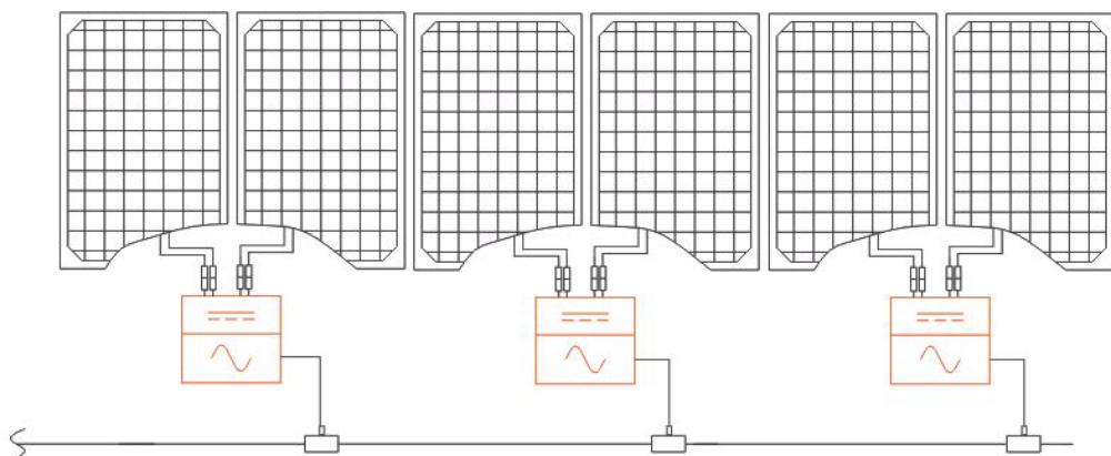
With its groundbreaking design and features, the YC600 is the pinnacle of microinverter technology. A single-phase, smart grid-compliant microinverter, the YC600 serves two modules with dual, independent MPPT. Zigbee wireless communication over a mesh network offers faster data speeds than PLC and a wider MPPT voltage range results in a greater energy harvest for homeowners.
